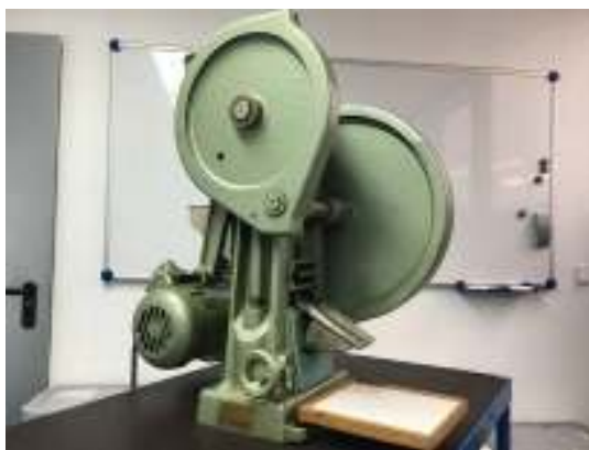
Figure 3: a. KORSCH tableting machine, Mod. 9341-72, Berlin. b. Special punches of Dome Matrix modules
