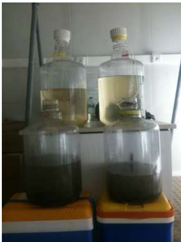
Figure 2. Seawater transport in the experimental tanks which followed the sediment transport. The use of silicone tubes was necessary to avoid any further disturbance and oxygenation in the experimental set-up.
