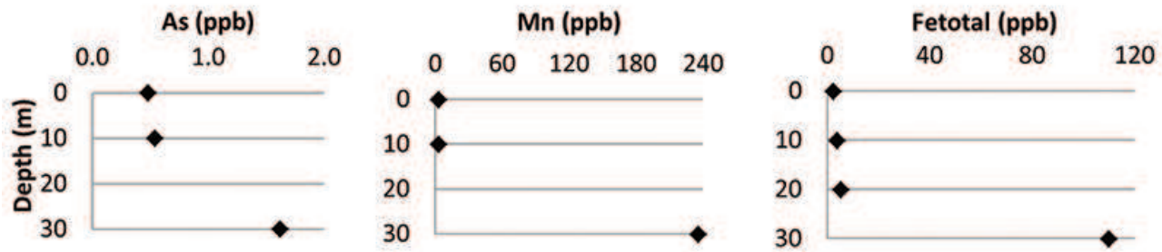
Fig.3: Total dissolvable As, Mn and Fe (ppb) for the water column of Elefsis Gulf
