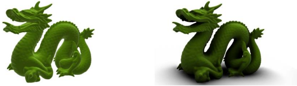
Figure 17: 3D model without ambient occlusion (left), and with ambient occlusion (right). The technique demonstrated is HBAO.
