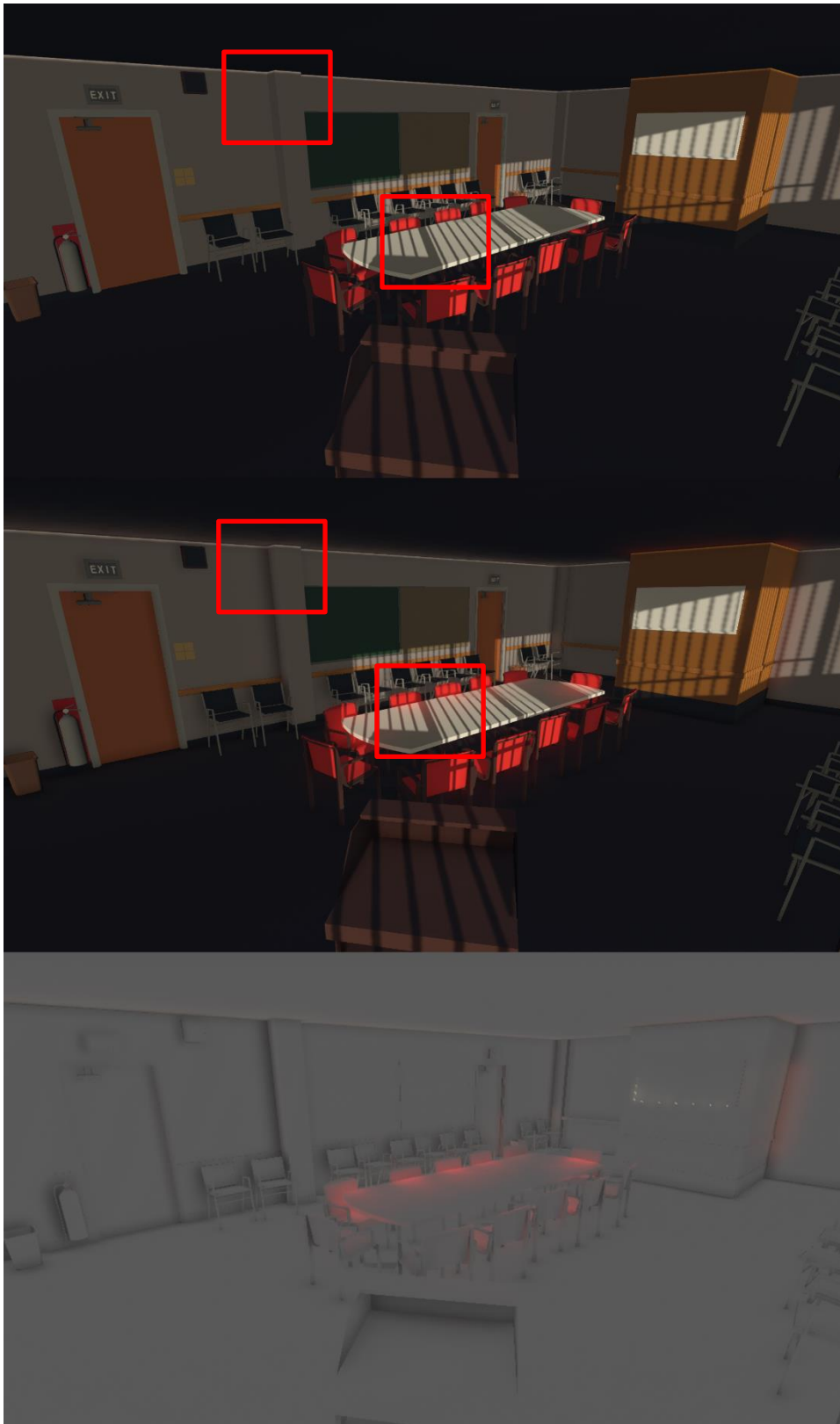
Figure 35: Conference room. From top to bottom: Scene without SSDO, scene with SSDO, SSDO debug view showing only the effect's contribution.
