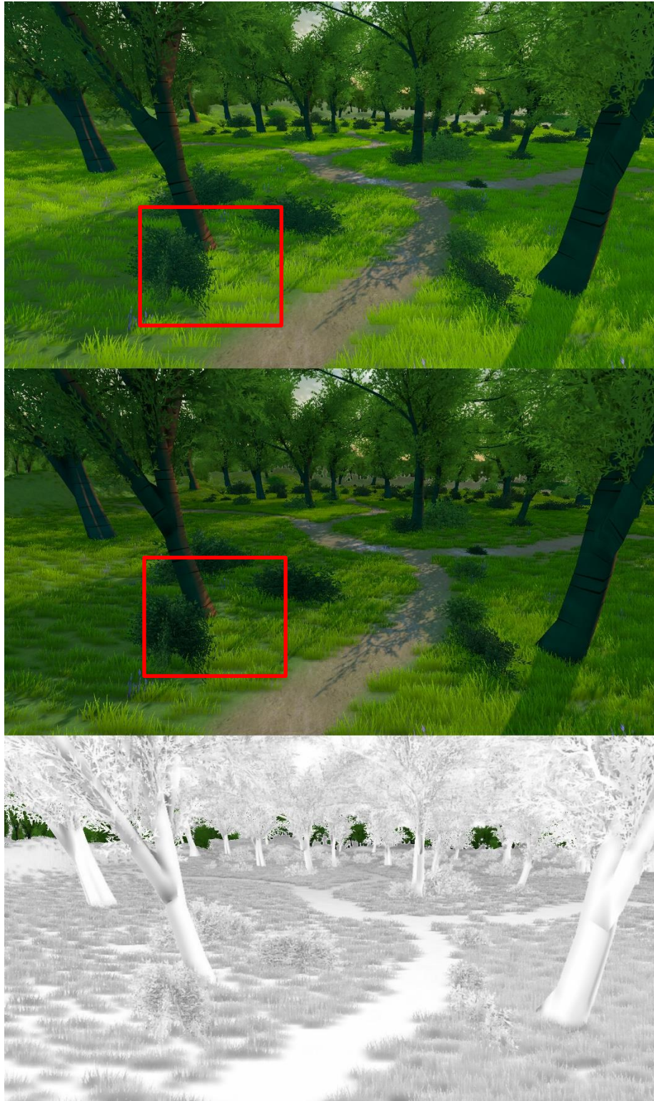
Figure 23: Forest scene. From top to bottom: Scene without SSAO, scene with SSAO, SSAO debug view showing only the effect's contribution.
