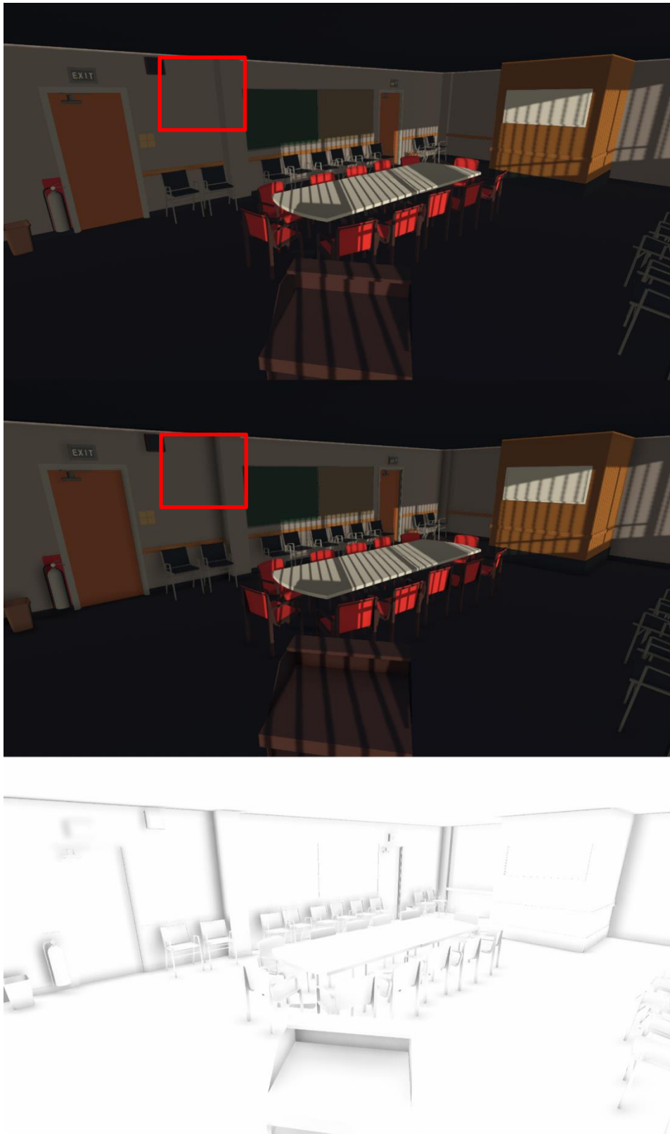
Figure 29: Conference room. From top to bottom: Scene without SSAO, scene with SSAO, SSAO debug view showing only the effect's contribution.
