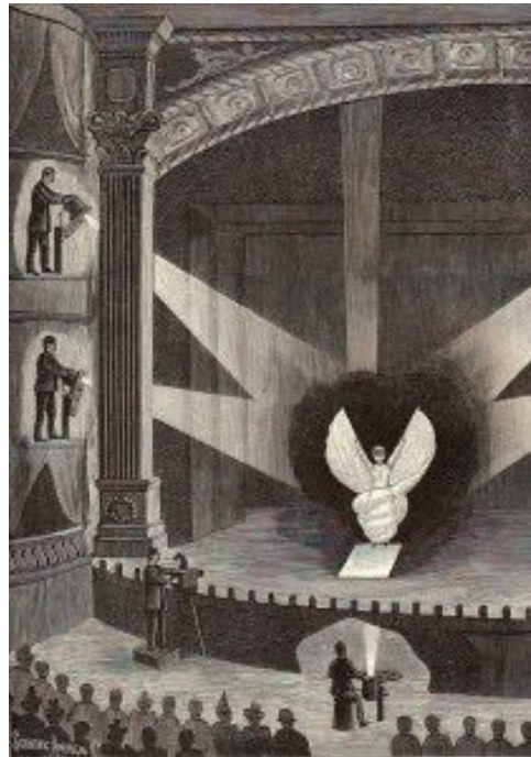
Figure 6: “An unauthorized illustration, originally published in “Scientific American” June 20, 1896, reveals the stage set-up for a Fuller-style dance. From Hopkins, Albert A., Magic: Stage Illusions and Scientific Diversions, including Trick Photography, Munn and Co., New York, 1901).”
