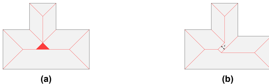
Figure 4: (a) 2D Voronoi diagram for polygon with colinear edges. (b) 1D Voronoi diagram after infinitesimal perturbation of edges, where \epsilon \rightarrow 0^+ .
