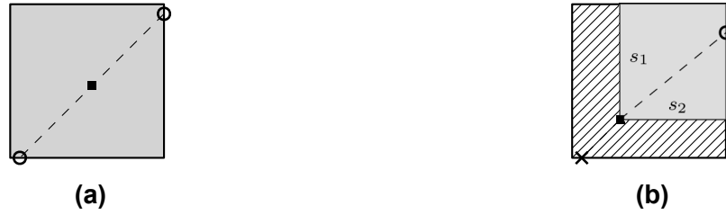
Figure 7: The intersection of the affine bisector and the cell. The circled points are in \mathcal{Z}^+(s_1) \cap \mathcal{Z}^+(s_2) , whereas the crossed point is not. Square nodes are the bisector nodes inserted to the output graph.
