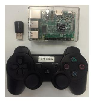
Figure 10: Raspberry Pi Model 3 B with case, wi-fi USB adapter and PlayStation3 controller.
