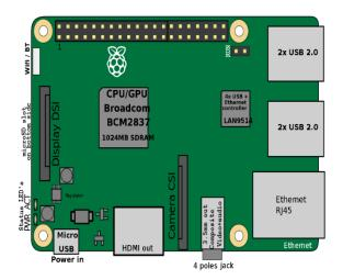
Figure 11: Raspberry Pi Model 3 B abstract architecture schema.
