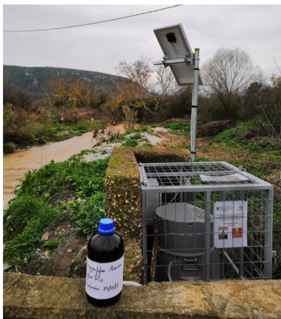
Figure 19: Autosampler near sampling point R2.
