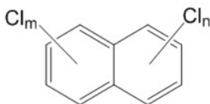
Figure 4: General structure of polychlorinated naphthalenes [15].
