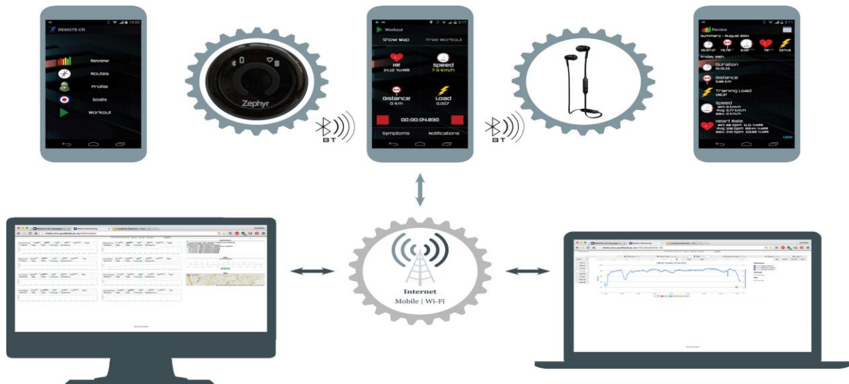
Figure 2: Remotely monitored exercise-based cardiac telerehabilitation platform schematic.
