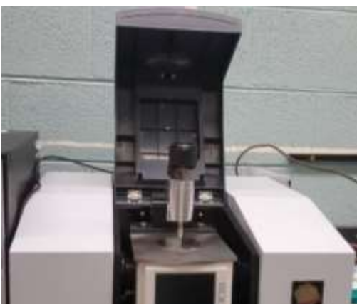
Figure 15: GladiATR Vision – Diamond ATR with Sample View. Spectral range is 4000–400 cm -1 with standard FTIR optics.
