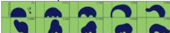
Figure 2. Simulation snapshots of droplet lateral movement on an inclined plane with air permeating the solid substrate.
