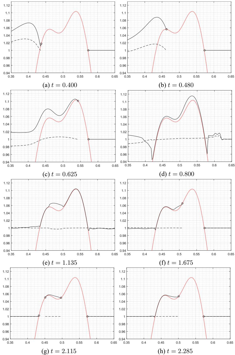
Figure 4.16: Flow over a complex bottom. Numerical solution ( $d + \beta$ : solid line,  $du+1$ : dashed lines,  $\beta$ : dotted lines, shore location: small circles) at various times.
