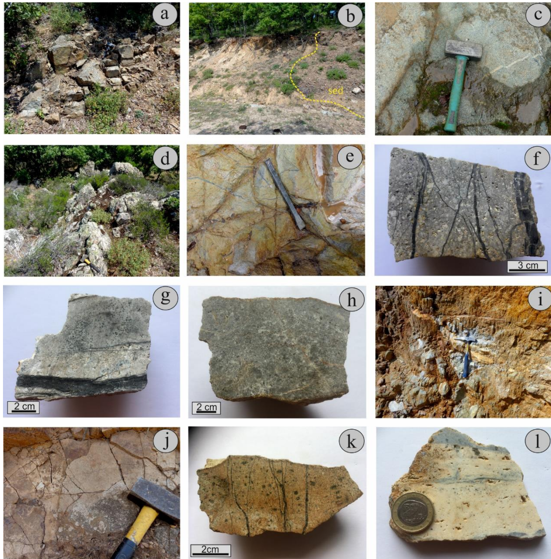
Figure 4.6: Field and hand-specimen photographs of porphyry/epithermal mineralization and alteration at the broad Sapes area. (a) Fresh to propylitic-altered granodiorite porphyry; (b) Marls unconformably overlying the sericitic-altered granodiorite porphyry; (c) Monzodiorite, slightly propylitized; (d) N10°W-trending microgranite porphyry dyke, close to Papadokoryphi hill; (e) Dense quartz porphyry stockwork, from the eastern slopes of Konos Hill; (f, g) Hand-specimen of quartz stockwork from Konos Hill. Note in g, the banded appearance of the vein and the pyrite center-line; (h) Sodic (albite)-altered granodiorite; (i) Gypsum vein (early anhydrite?) with base metal mineralization; (j,k) Weak quartz porphyry stockwork
