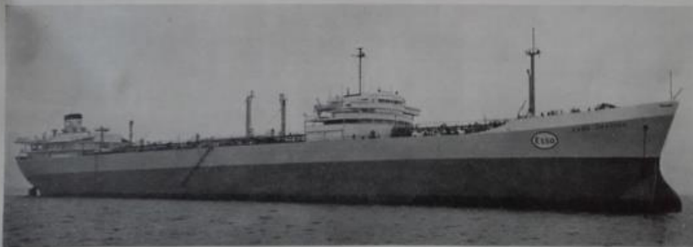
The lengthened tanker "Esso Jamaica" clearly showing the addition of the bulbous bow
