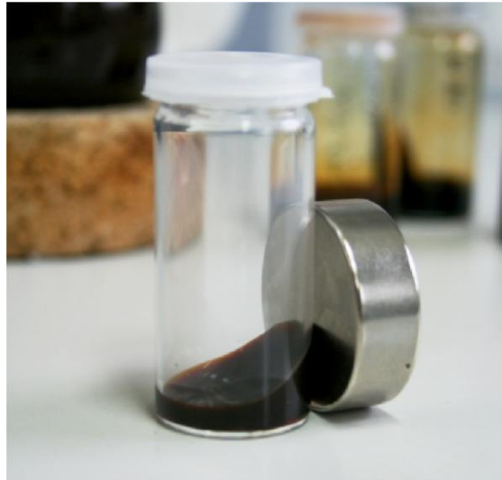
Figure 8. Fluidal sample of Magnetic nanoparticles, synthesized at the Institute of Medical Engineering of the University of Lübeck, magnetized by a permanent magnet [PAN15].
