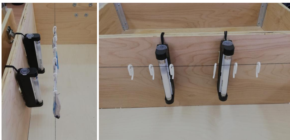
Fig. 58 Handmade photocatalytic apparatus for the case of fabrics.
