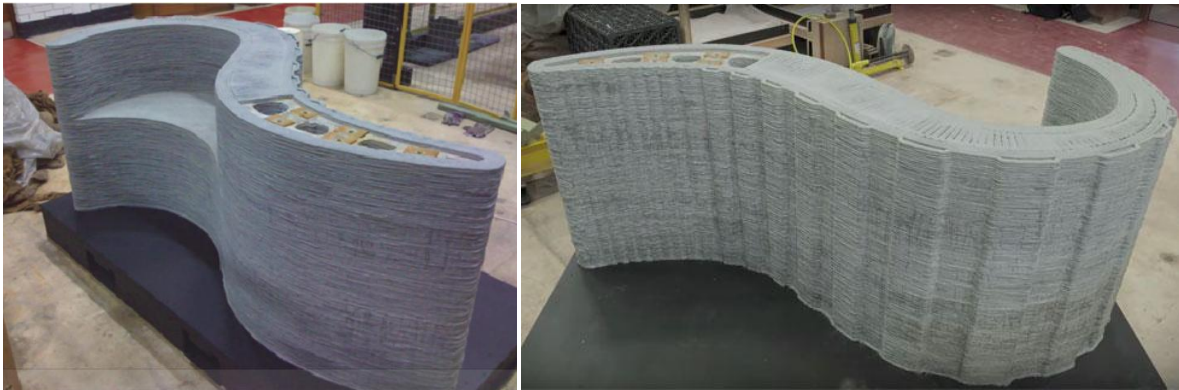
Fig. 35 Wonder bench constructed by Concrete Printing. [S. Lim et al., 2012]
