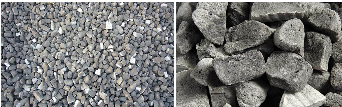
Fig. 41 Foamed glass gravel. [Geocell]
