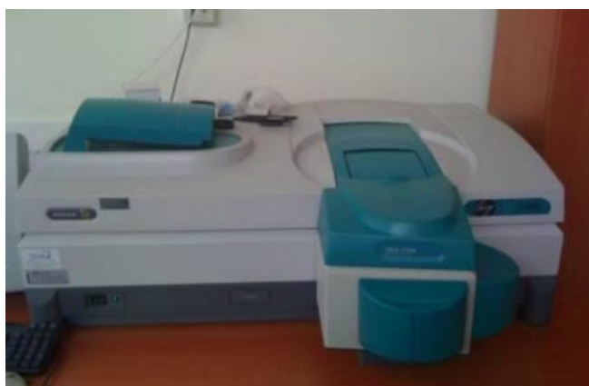
Fig. 56 Color coordinates of CIELAB model and Varian CARY-5000 DRA 2500 UV-VIS-NIR Spectrophotometer. [Sappi]
