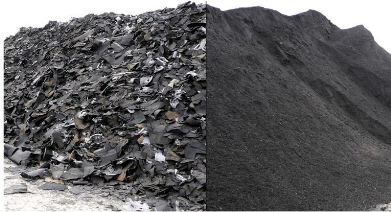
Fig. 43 Asphalt Shingles before (left) and after (right) recycling. [J.N. Davis Roofing Co.]
