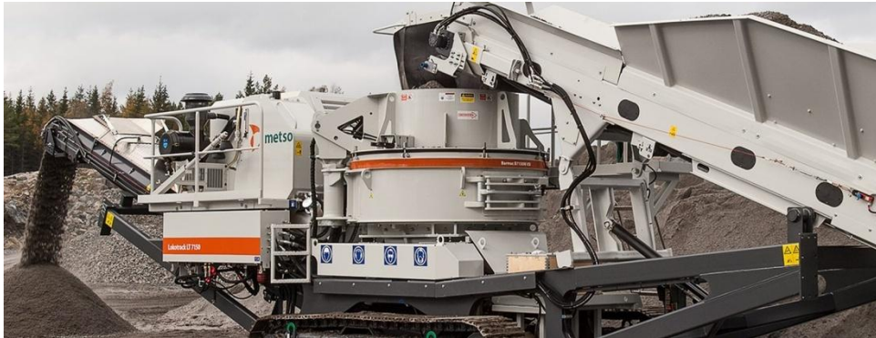
Fig. 49 Mobile vertical shaft impact (VSI) crusher plant. [Metso-Impact]
