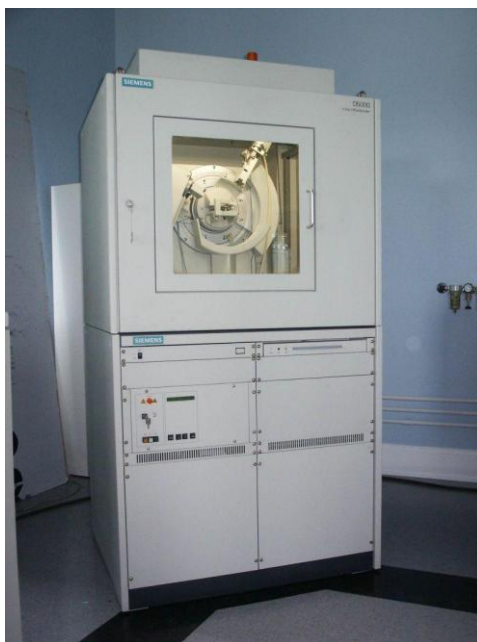
Fig. 52 Siemens D5000, X-ray diffractometer. [LabX]
