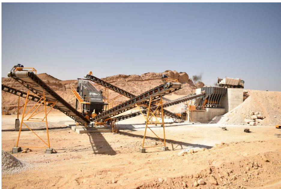
Fig. 46 Stationary crusher plant. [Fabo-Stationary]
