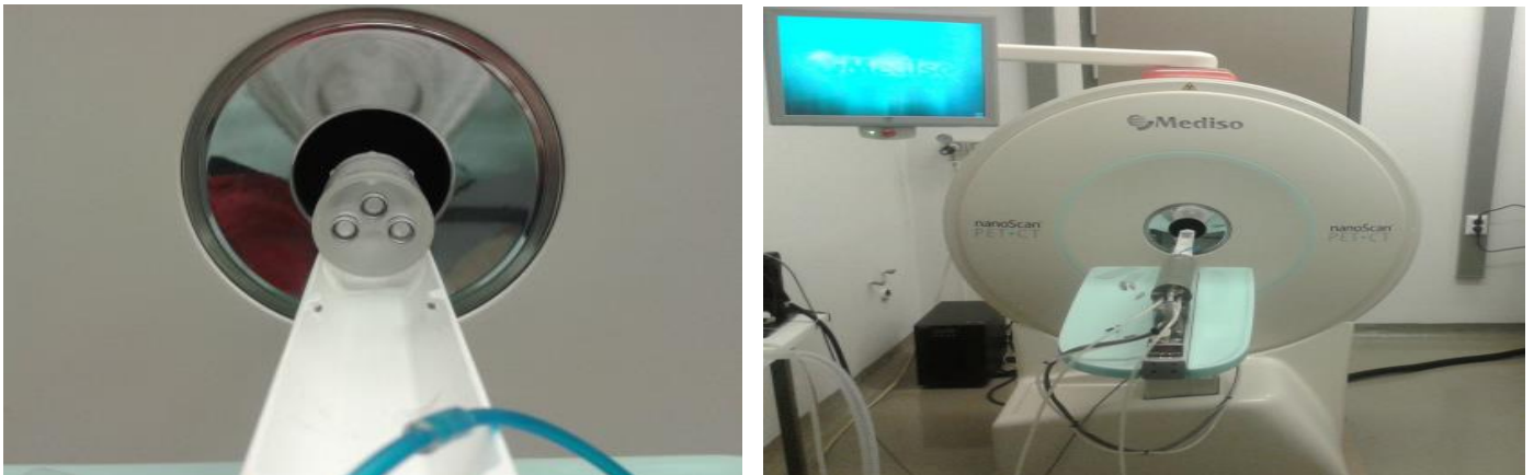
Figure 14. Images from the front and anterior side of the Mediso NanoScan ® PC. In the first image, the IQ phantom which was used in the studies, can be seen.
