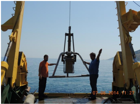
Figure 3.2. Box corer deployment for sediment sampling (left photo) and box corer recovery (right photo) on board R/V “Aegaeo”.
