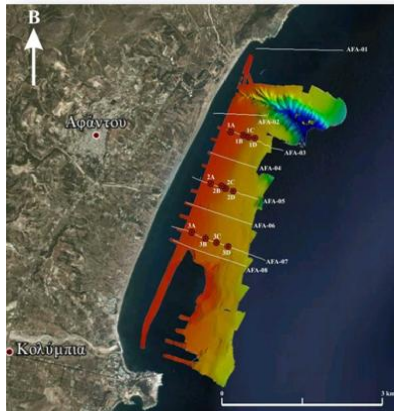
Fig. 5.60. Bathymetry, seismic lines and sampling positions in the Afantou Bay (Kapsimalis et al., 2013).
