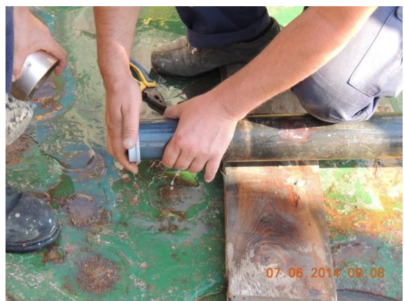
Figure 3.6. Gravity core sampling on board R/V “Aegaeo” and suitable preparation for safe transfer at the laboratories.
