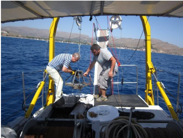
Figure 3.14. Smith-McIntyre grab filled with sediment sample on board R/V “Alkyon” (left photo) and sample L-E8 collected from the offshore area of Eresos with Smith-McIntyre grab (right photo).
