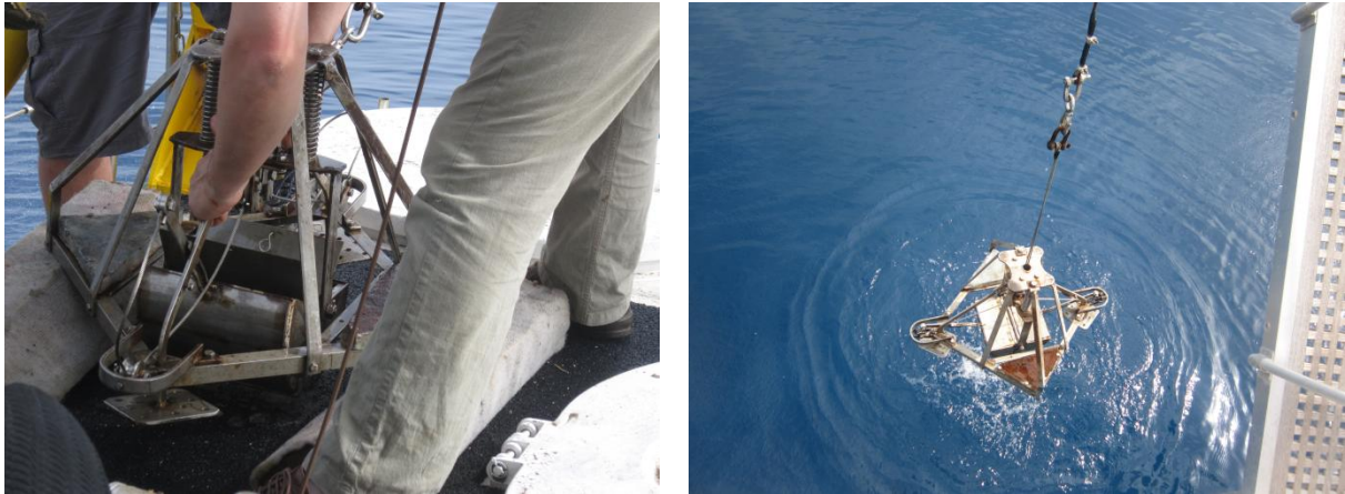
Figure 3.9. Smith-McIntyre grab preparation for sediment sampling (left photo) and Smith-McIntyre grab recovery filled with sediment sample (right photo) on board R/V “Alkyon”.
