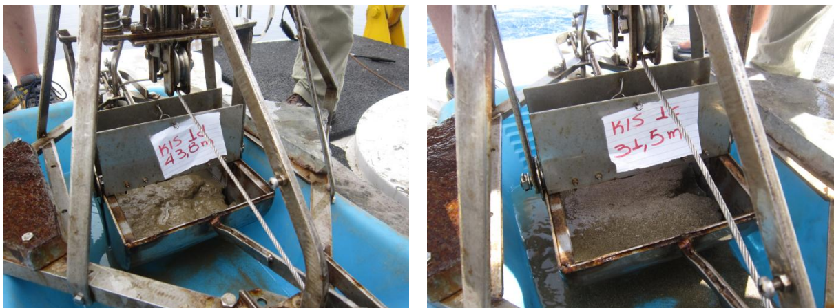
Figure 3.10. Sample KIS-1D with fine material (left photo) and sample KIS1C with coarser (sand) material (right photo) collected with Smith-McIntyre grab on board R/V “Alkyon”.
