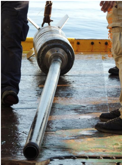
Figure 3.5. Gravity core sampler after a failed attempt (left photo) and gravity core ready for sampling (right photo) on board R/V “Aegaeo”.
