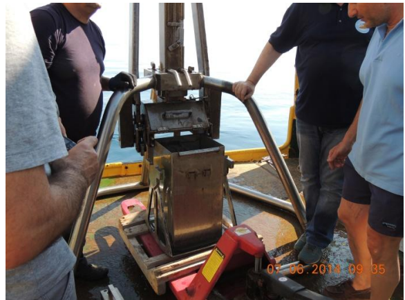
Figure 3.2. Box corer deployment for sediment sampling (left photo) and box corer recovery (right photo) on board R/V “Aegaeo”.
