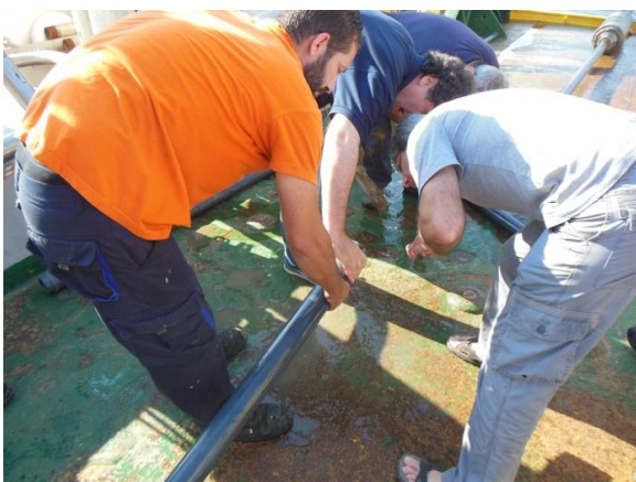
Figure 3.6. Gravity core sampling on board R/V “Aegaeo” and suitable preparation for safe transfer at the laboratories.
