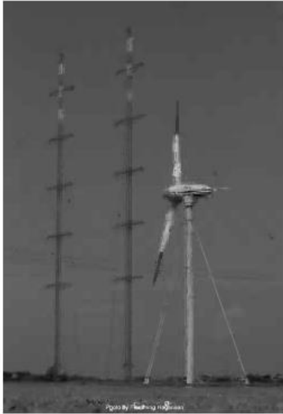
Figure 15: The 3-MW Growian HAWT near Bremerhaven, Germany. It was one of the largest wind turbines ever built, with a 100-m diameter rotor and a 100-m tall tower 38
