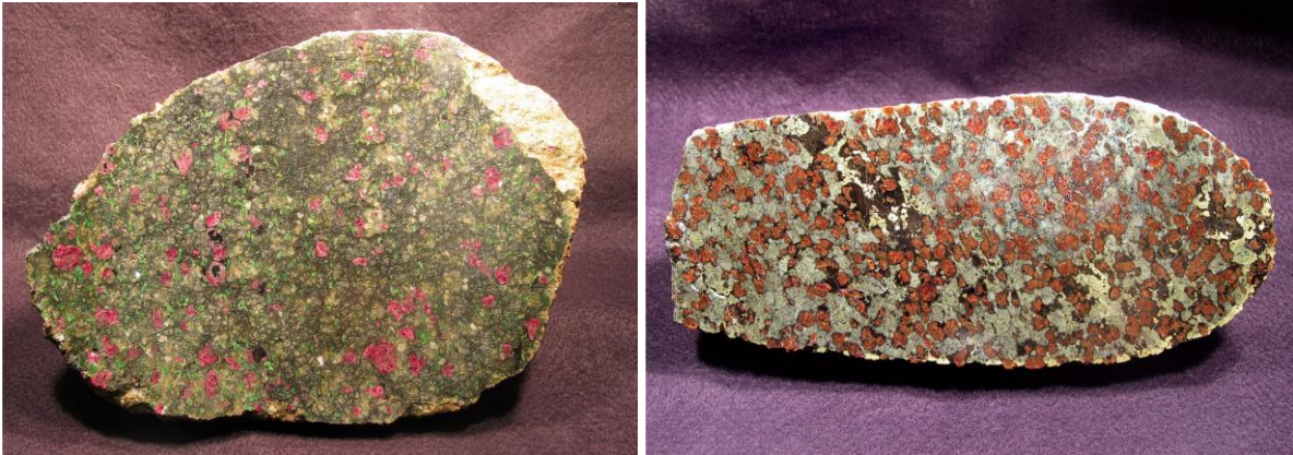
Fig. 6. On the left , a piece of peridotite xenolith from the Bultfontein mine, Kimberley, South Africa (diameter \sim 30 cm), which consists mainly of olivine (dark green), garnet (purplish red), Cr-diopside (bright green), and orthopyroxene (light brown). On the right , a piece of eclogite xenolith from the Roberts Victor mine, South Africa (diameter \sim 30 cm), which consists mainly of garnet (reddish-brown) and clinopyroxene (grayish-green). Eclogites are a minor constituent of the lithospheric mantle, but they can be important diamond source rocks.
