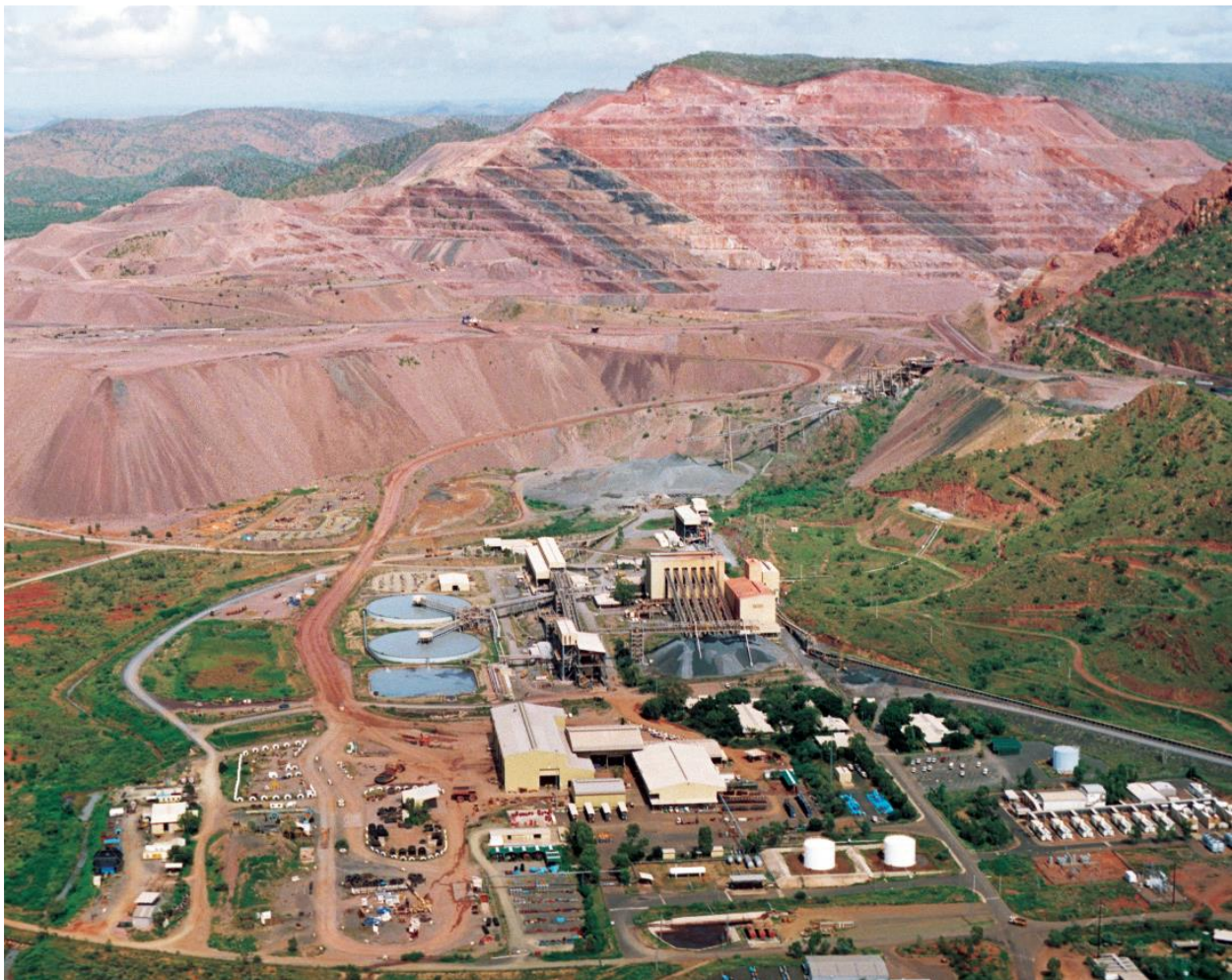
Fig. 8. Aerial view of the Argyle diamond mine, Western Australia, showing processing plant, tailings piles, and tilted sedimentary rocks of Proterozoic age, which form the wall rocks of the mine. (From Tappert & Tappert, “Diamonds in Nature – A guide to rough diamonds”, 2011, their figure 1-15)
