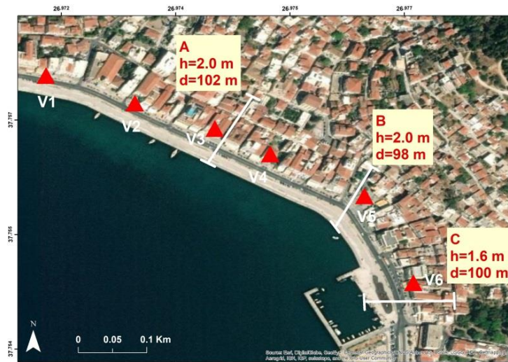
Figure 8.10. Observation sites V1 to V6 (red triangles) along the Vathy bay east coast and three characteristic tsunami transects A,B,C (white lines) measuring maximum run-up, h , at respective run-in distance, d (for details see in text).
