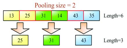
Figure 3.1: MaxPooling1D layer.
