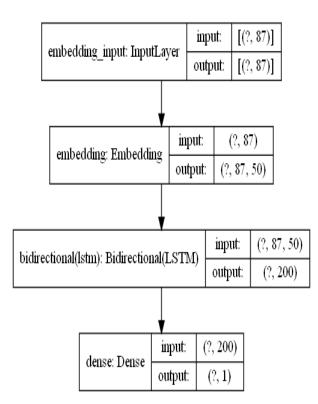
Figure 3.3: LSTM model for tweet classification.
