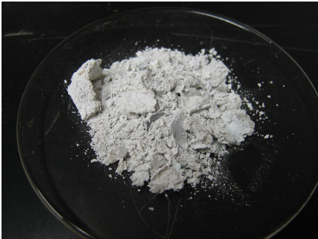
Figure 2: The flakes of crude lead white scraped from the residual piece of lead. Author's laboratory
