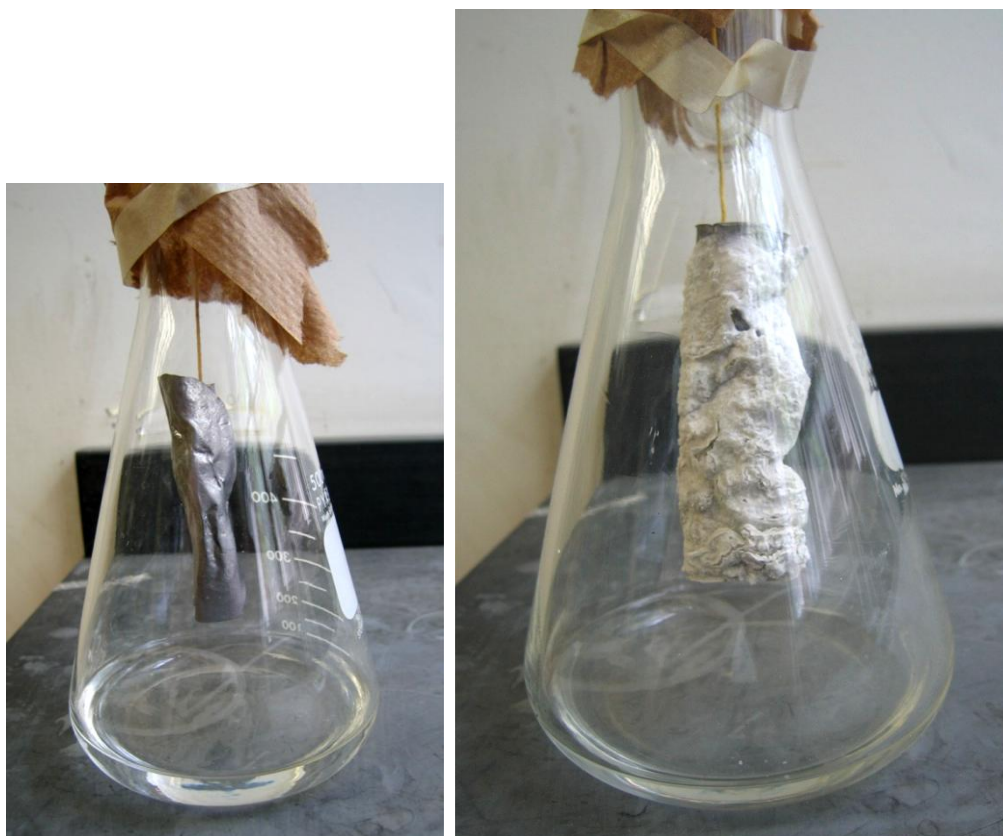
Figure 1: Before and after photographs of the lead white experiment; at the start of the experiment (left) and after twenty days (right). Author's laboratory
