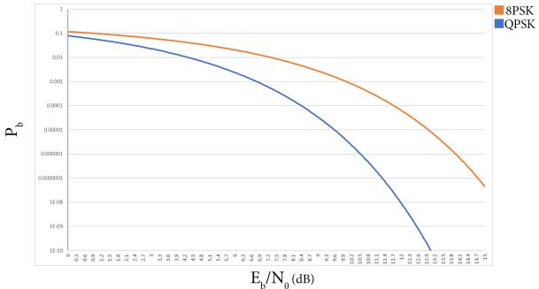
Figure 4.17 – Bit-error probability  $P_{h}$  vs SNR per bit  $E_{h}/N_{o}$  in AWGN conditions
