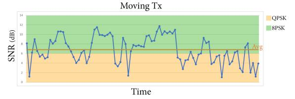
Figure 4.14 – SNR estimations over time for moving transmitter
