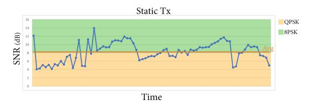
Figure 4.13 - SNR estimations over time for static transmitter
