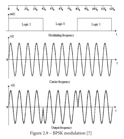
Modulator operations for BPSK are rather simple. Given a bipolar NRZ baseband modulation as displayed in (13), the resulting signal for a sinusoidal carrier can be written as (14).
