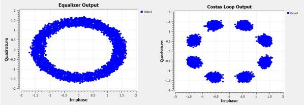
Figure 4.4 – QT GUI Constellation Sink display at CMA Equalizer and Costas Loop outputs. Slight frequency offset and noise are applied.
