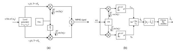
Figure 2.13 – MPSK (a) modulator and (b) demodulator block diagrams [4] the constellation space. Its probability density function is two-dimensional, bell-shaped, centered at
