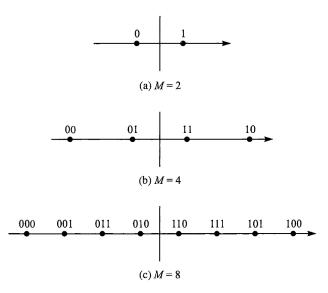
Figure 2.7 – M-PAM Constellation for (a) M=2 (b) M=4 and (c) M=8 [3]
