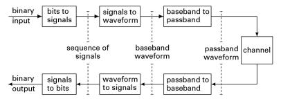
Figure 2.1 - Simple signal processing chain block diagram [2]
