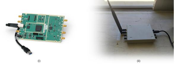
Figure 3.6 – USRP B210 (i) Board only [21] (ii) Complete with enclosure and antennas, used in lab
