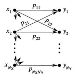
Figure 2.4 – Discrete Memoryless Channel Model [6]
