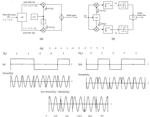
Figure 2.11 - QPSK (a)modulator, (b) demodulator block diagrams, parallel pulse streams, signal components and transmitted signal waveforms [4]
