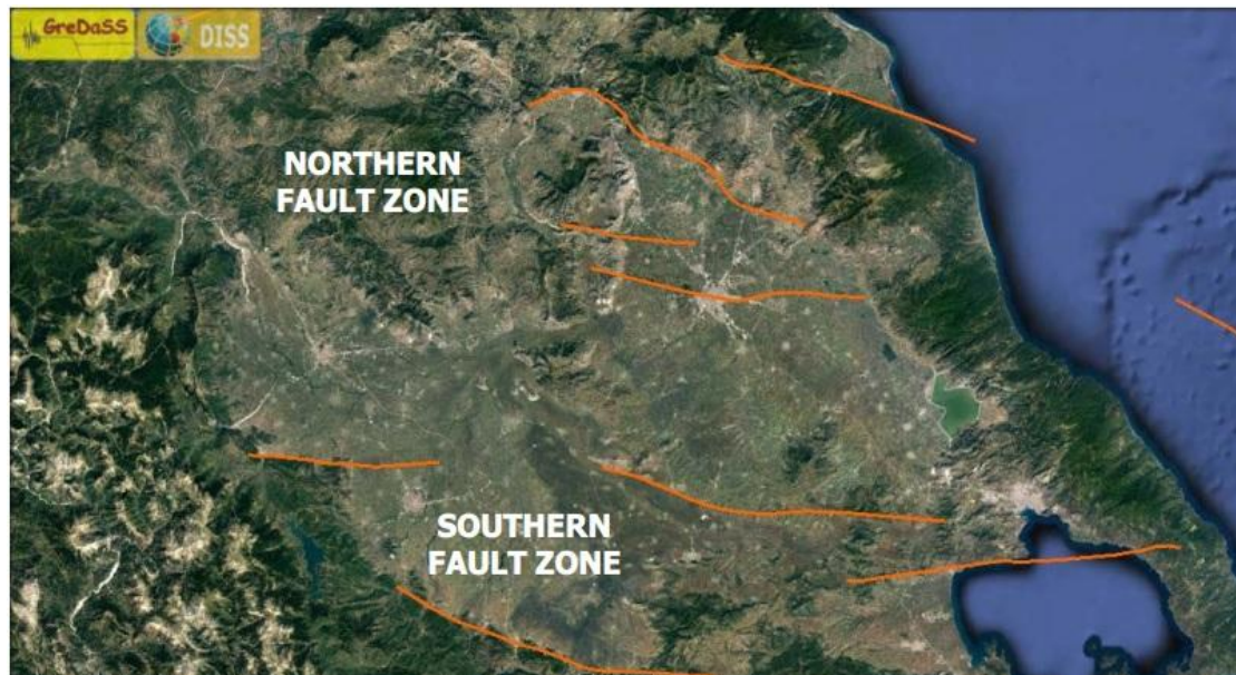
Figure 2: The two fault zones: the northern fault zone, which is associated with earthquakes with magnitudes up to 6.5 and the southern fault zone associated with earthquakes with magnitude up to 7.0 (Lekkas E. et al., 2021).
