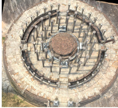
Figure 8: Medirigiriya Vatadage – 3 circles of columns (Zamani Project)
