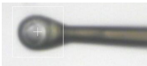
Figure 7.10: Crystal of M2(22-46) V27A during data collection. Loop diameter is 35 \mu\text{m} ; crystal is visible as a thin rectangular plate inside the loop.
