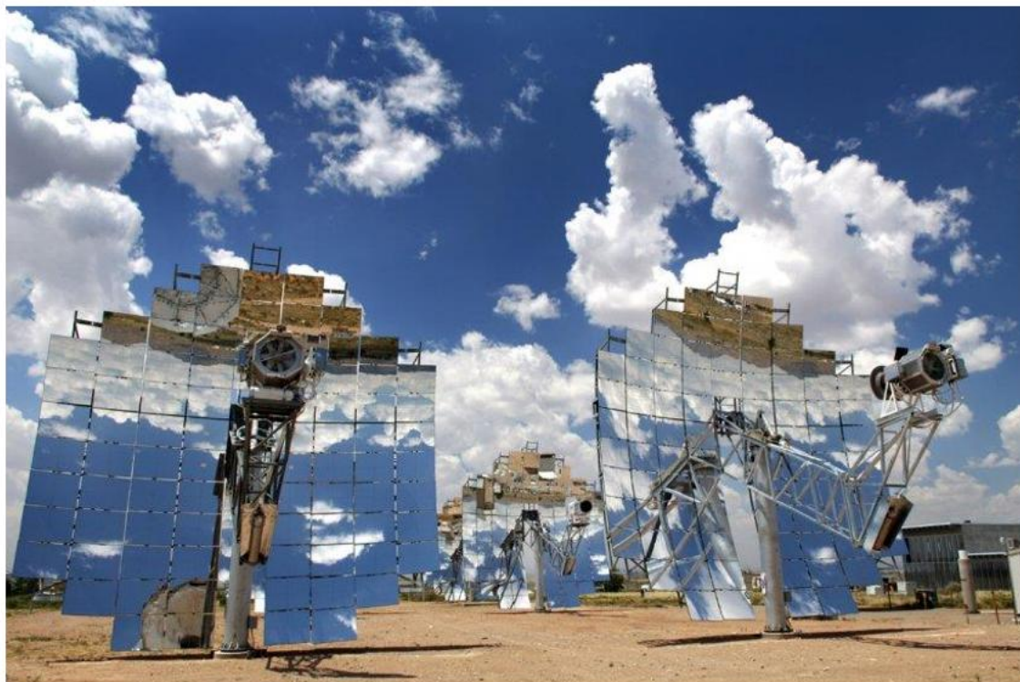
Εικόνα 127: Dish Stirling - Concentrated Solar Power (Energy Efficiency & Renewable Energy- Solar Dis Sets World- Record Efficiency)
