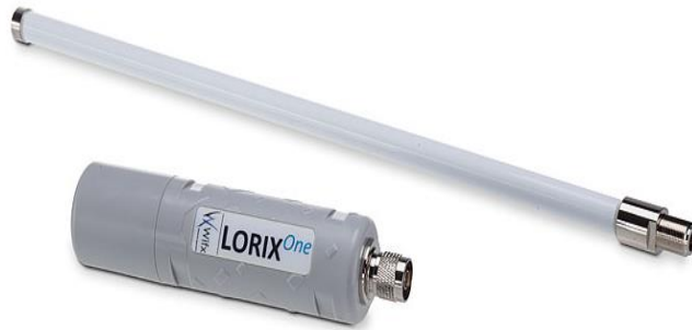
Figure 3: The LORIX One gateway
