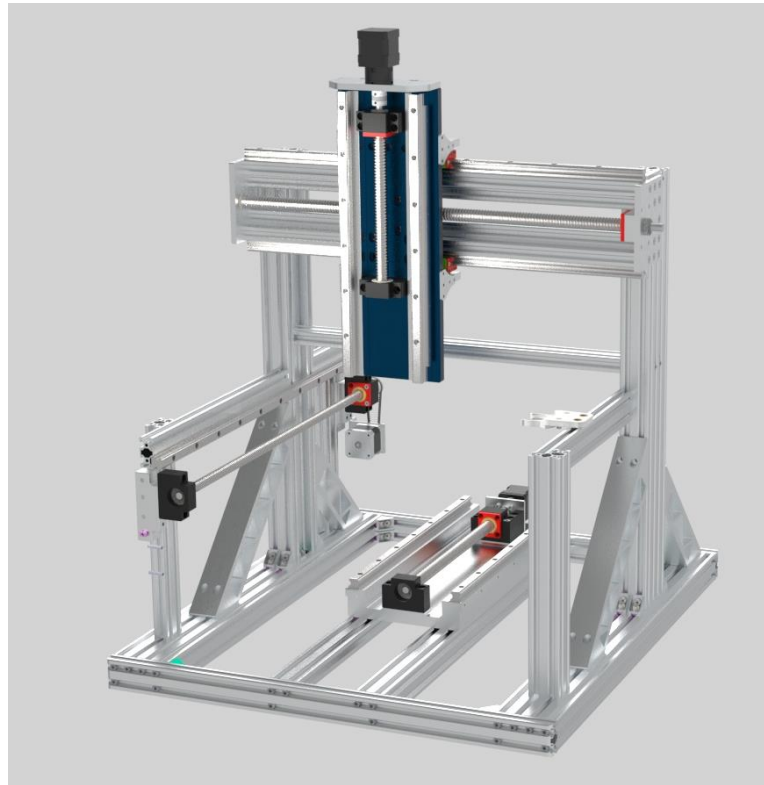
Figure 5: The proposed 5-axis hybrid CNC frame.
