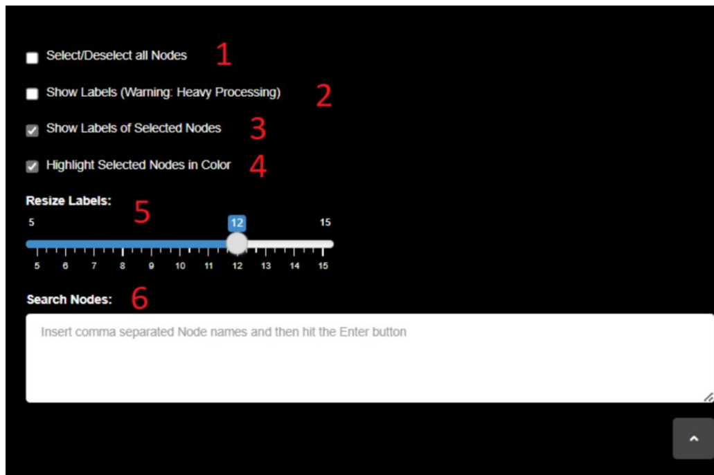
Figure 8.7 “Node Actions” menu option in Arena3Dweb. 1. This option allows the user to select/deselect all nodes. Selected nodes can then be translated in 3D space via the Navigation Controls, and via the Layer Selection & Layouts action tab can be either rearranged in a local layout or rescaled based on network metrics. 2. This option allows the user to view every node label. This is an option that demands heavy processing power due to the constant redrawing of labels. Ensure that this is enabled only in small networks and in combination with the 15FPS option of the FPS action tab. 3. This option allows viewing only the labels of selected nodes. Priority is given in option (2) over this option. 4. Selected nodes are highlighted in a chartreuse color. Deselecting this option allows nodes to retain their original color (either from any uploaded node attributes or from their default layer color). Deactivating this option works in combination with activating option (3), to select certain nodes of a pre-colored path, view their labels without changing their color and extracting the respective image (either with the PrintScreen key, or by snipping or by right-clicking and then selecting the Save as Image option). 5. This option allows resizing of node labels. 6. This is the node search bar. The user can select multiple nodes by entering their names, without the need to specify layers, separated by commas. Any trailing and leading spaces are trimmed.
