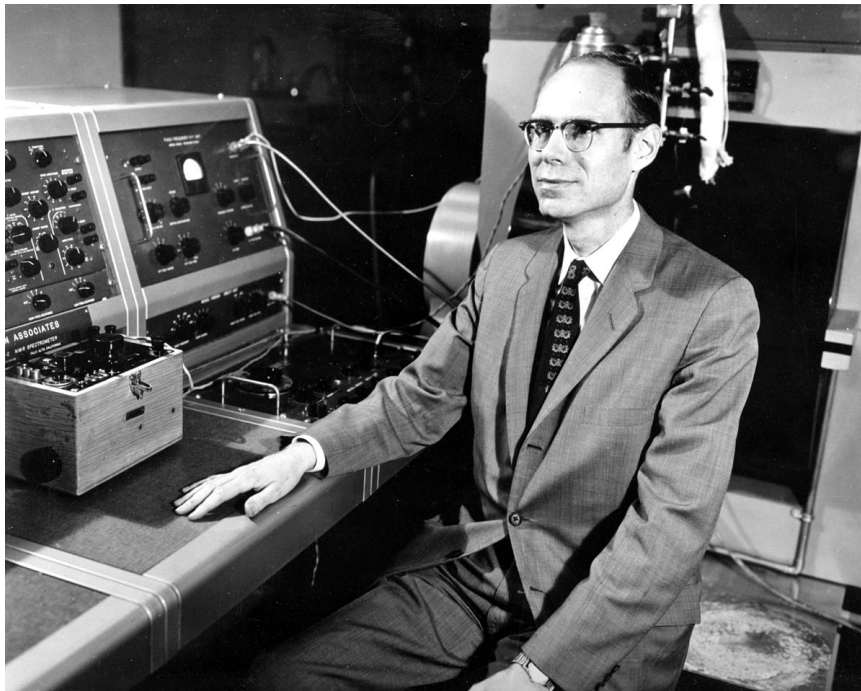
Figure 1: 1952 - AUDREY - Bell Labs. A six foot high rack of supporting analog-circuitry electronics is not shown.
