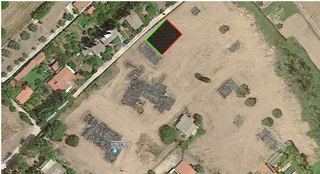
Figure 1.4: Satellite image depicting the area where the GPR survey took place (displayed with a rectangle). The starting and the ending points of each GPR profile are presented with green and red colour respectively. (Google earth).
