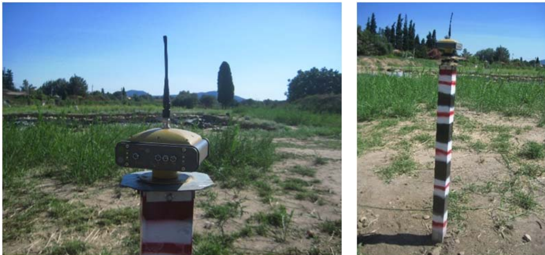
Figure 1.7: Topographic reference Base set near the area of interest.
