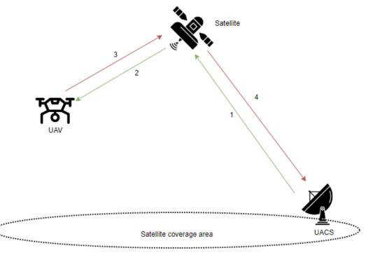
Image 54: Links for BLoS with satellite as relay
