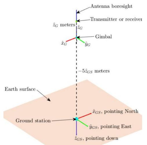
Image 37: Cartesian coordinates for both gimbal and transmitter/receiver for the ground station [65]
