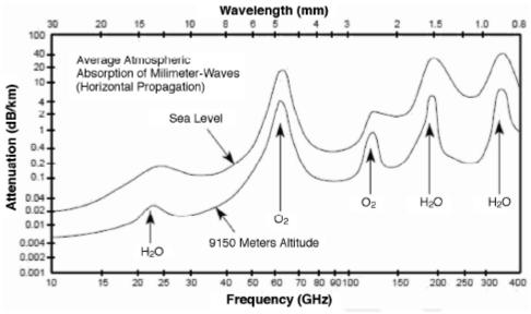
Figure 8: Atmospheric loss relative to frequency and wavelength [72]
