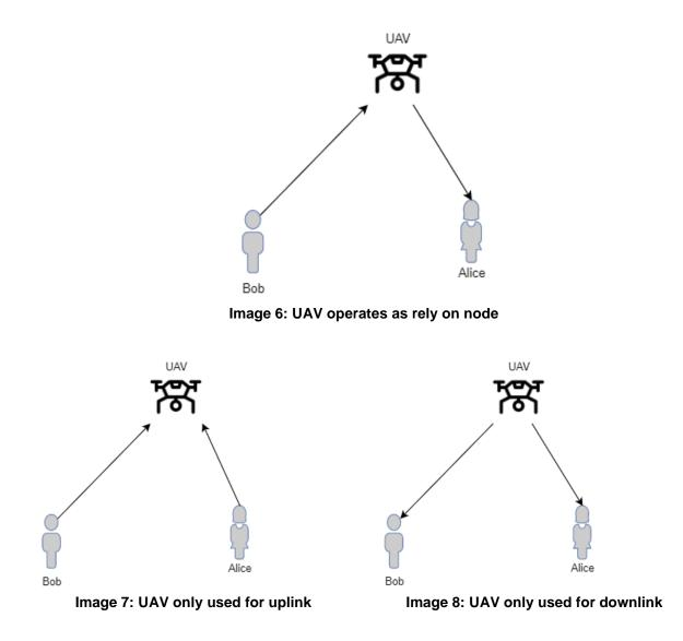
Both Image 7 and Image 8 show the one-way communication between a terrestrial entity and an aerial vehicle. The first one supposes that UAVs are only used to receive data that are stored locally, while the latter one only transmits data to specific entities. The difference between Image 8 and Image 9 is that the last one multicast the message to everyone in the coverage area and not to specific users, thus if a  $3^{rd}$  person was in the coverage area, could normally receive the UAV data.
