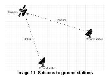
The above Figure gives an idea about ground communication. For example, one ground station may be in Australia, while the other one is in the USA and because they are in BLoS communication they transmit/receive data through a satellite. Uplink is called the channel where a ground station is transmitting traffic and downlink when the entity is receiving traffic data.
