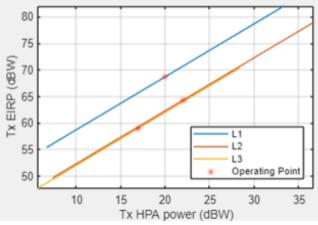
Figure 11: EIRP and HPA power comparison
