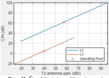
Figure 25:  $C/_N$  relative to transmitting antenna gain
