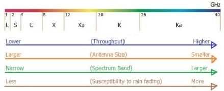
Image 10: Frequency bands and basic features of satellite communication [11]
