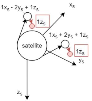
Image 36: Transmitter and receiver cartesian coordinates
