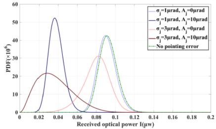
Figure 6: PDF for both pointing and no-pointing error for downlink channel
