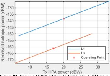
Figure 21: Received EIRP relative to transmitted HPA power
