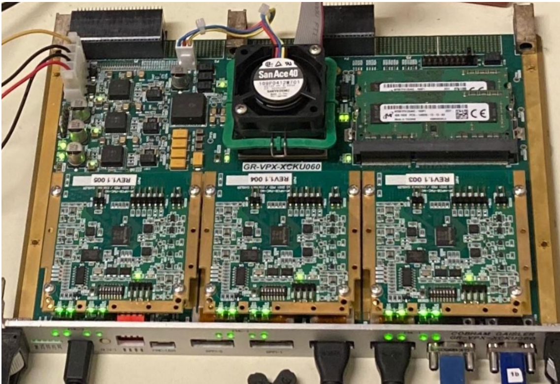
Figure 6.9: The evaluation setup with the GR-HPCB-FMC-M2 mezzanine card combined with the GR-VPX-XCKU060 carrier board.
