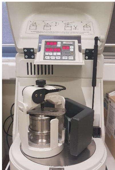
Figure 36: Principle of operation of planetary ball milling (top left) and SPEX ball milling (top right). 321 Planetary ball mill with jar (bottom left). SPEX mill (a) and tungsten carbide jar with spheres (b) (bottom right). 198
