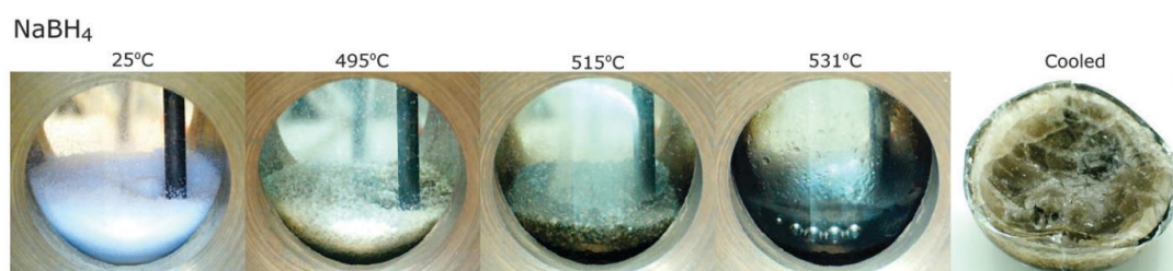
Figure 15: Photographic sequence of \text{NaBH}_4 thermal decomposition at 10 °C/min under 1 bar of \text{Ar} . 147
