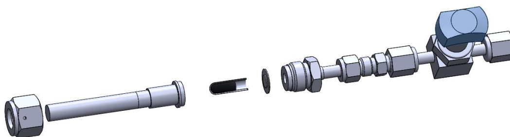
Figure 37: 3D model of the stainless-steel reactor used to perform the borohydride infiltration into the carbon scaffolds and the sorption cycling experiments on the samples.
