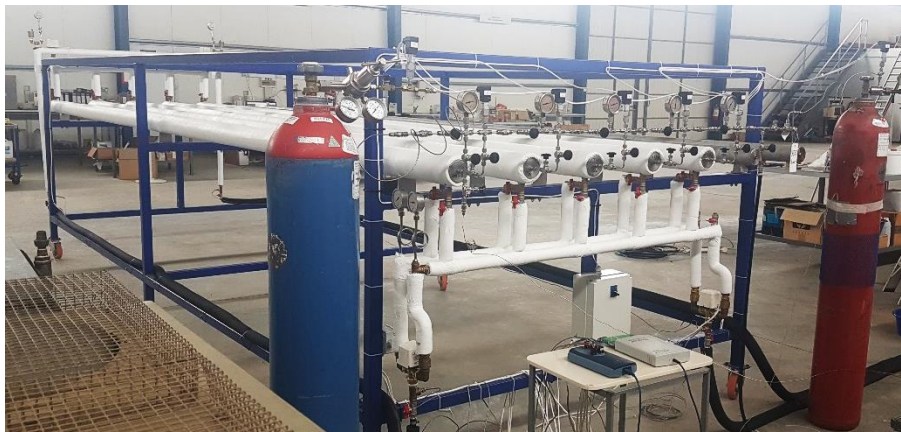
Figure 4: Prototype of a metal hydride compressor built in the framework of the ATLAS project in Hystore Tech (CY).
