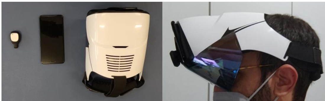
Figure 6: Low-cost equipment of the HOLOBalance platform. Inertia measurement unit, mobile phone, head mounted display. Cumulative weight: 583 gr.
