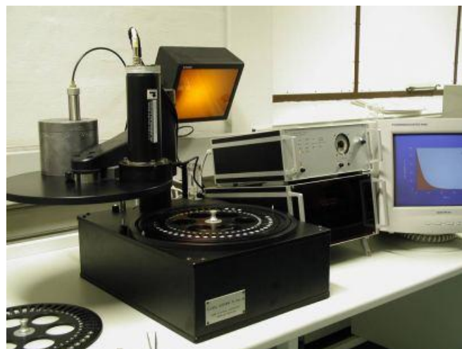
Figure 10 A laboratory model of the combined TL/OSL reader developed by Risø National Laboratory. Source: https://sci.esa.int/web/sci-fmp/-/40503-optically-stimulated-luminescence-dating-osl
