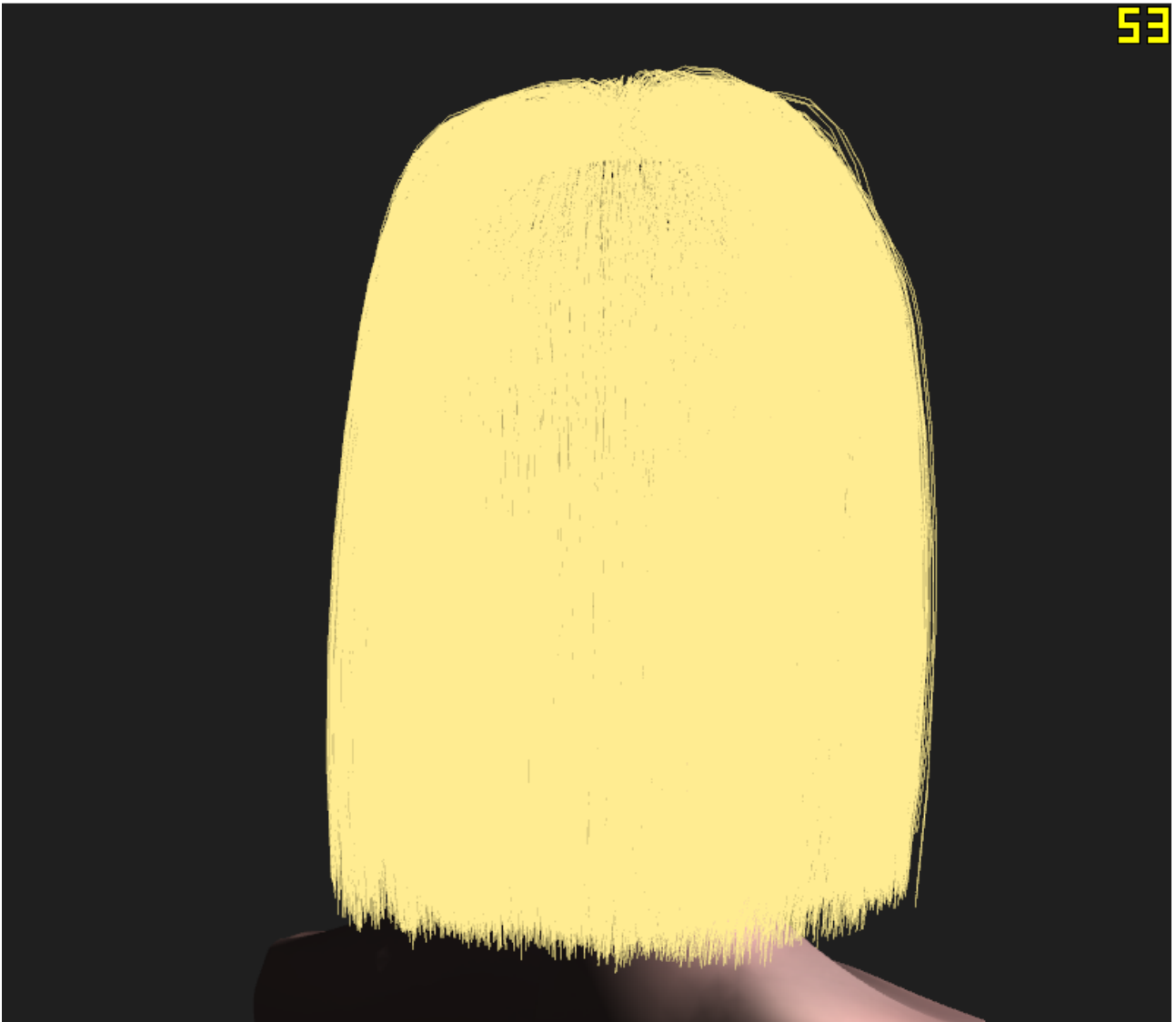
Figure 3.2: Rendering a hairstyle by sending every strand to the GPU. This is a performance bottleneck
