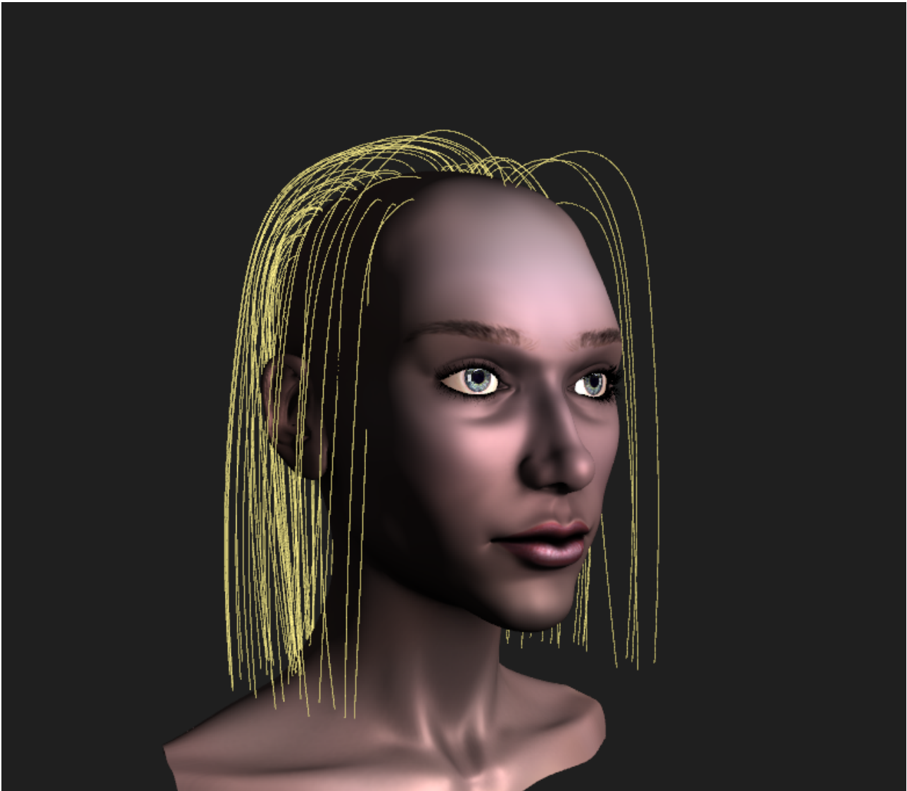
Figure 6.3: Rendering the guide strands as cubic b-splines using hardware tessellation.
