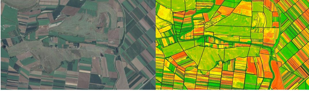
FIGURE 1.10: Raw corn field image (left) vs its NDVI counterpart (right) (Smart AKIS)
