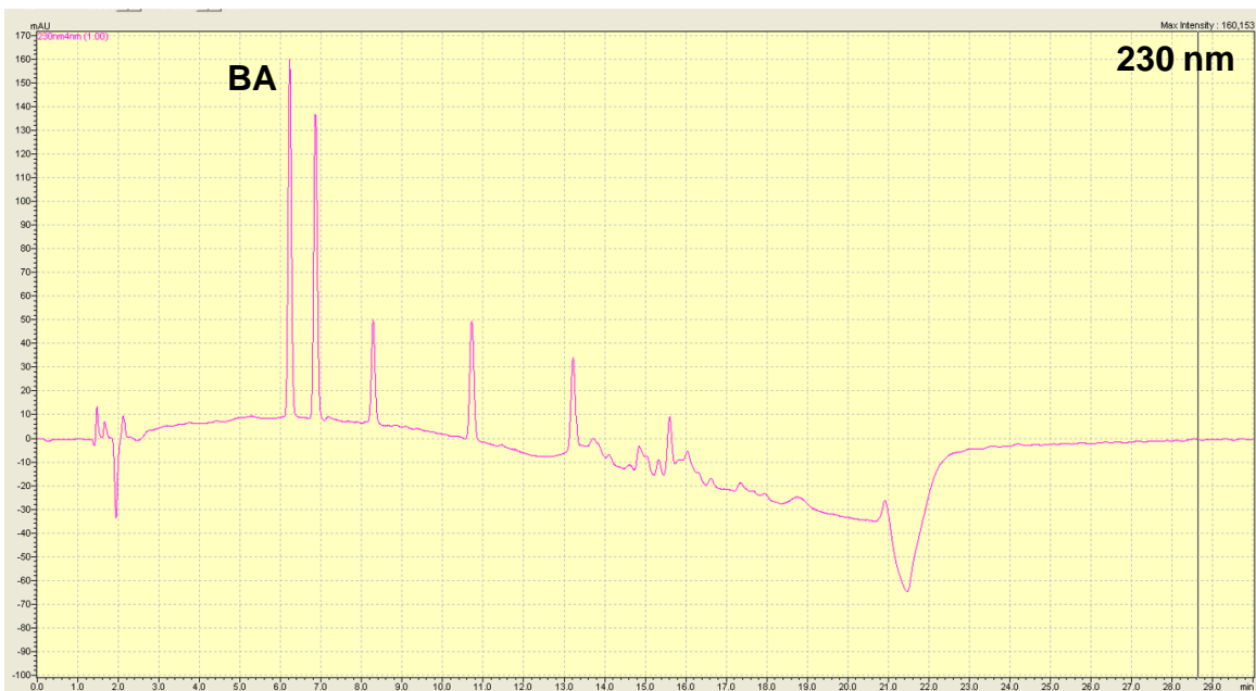
Figure 24: Chromatogram of Mix standard (10 µg/mL in 20:80 ACN:H 2 O), Elution Program 7, Flow rate: 1 mL/min, 230 nm.
