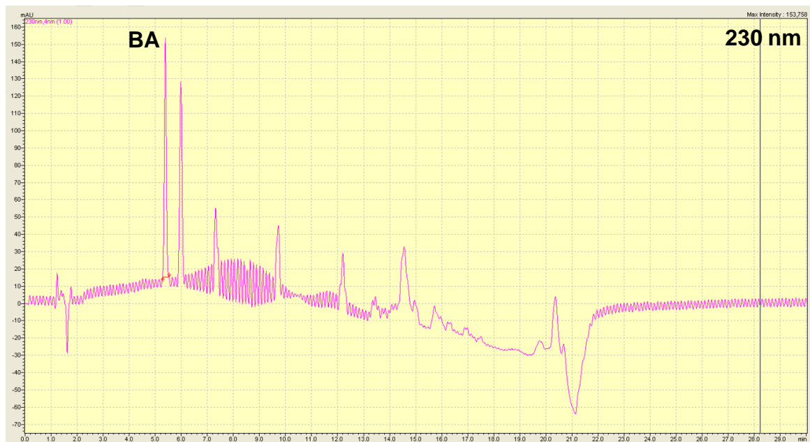
Figure 26: Chromatogram of Mix standard (10 µg/mL in 20:80 ACN:H 2 O), Elution Program 7, Flow rate: 1.2 mL/min, 230 nm.
