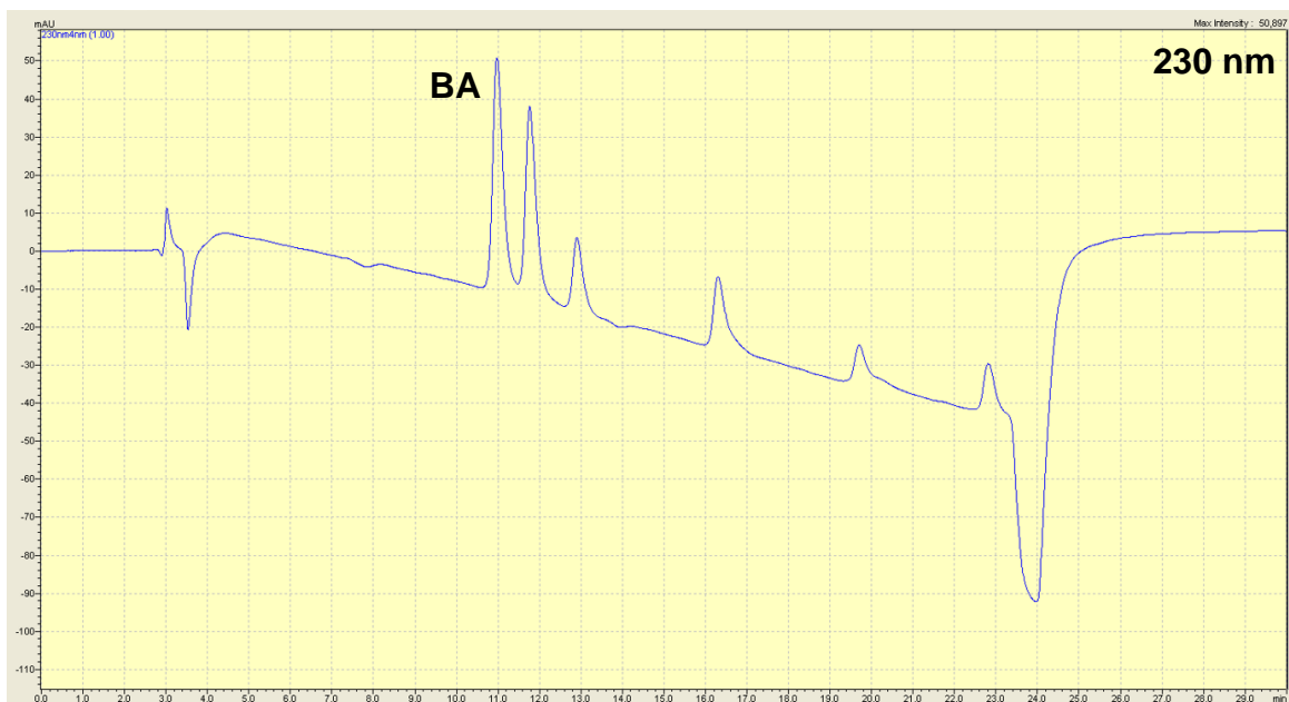
Figure 12: Chromatogram of Mix standard (10 \mu\text{g/mL} in 50:50 MeOH:H 2 O), Elution Program 2 in 230nm.
