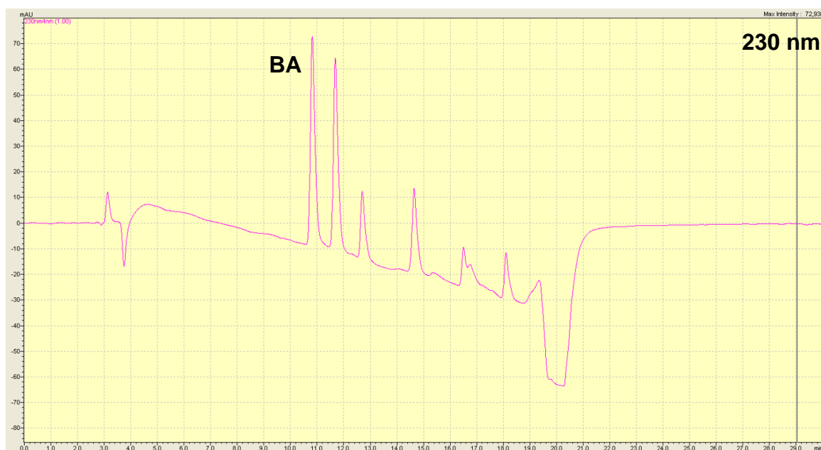
Figure 16: Chromatogram of Mix standard (10 µg/mL in 50:50 MeOH:H 2 O), Elution Program 4 in 230 nm.
