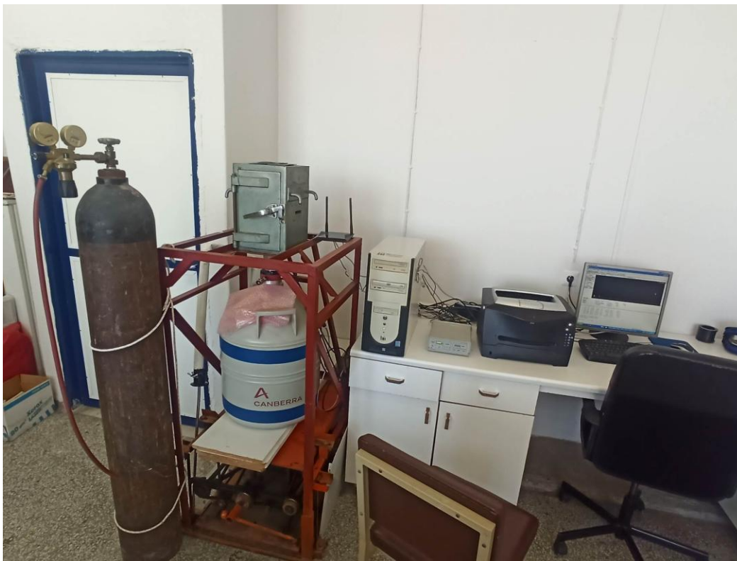
Figure 7: The \gamma -ray Spectroscopy system used in radioactivity measurements.
