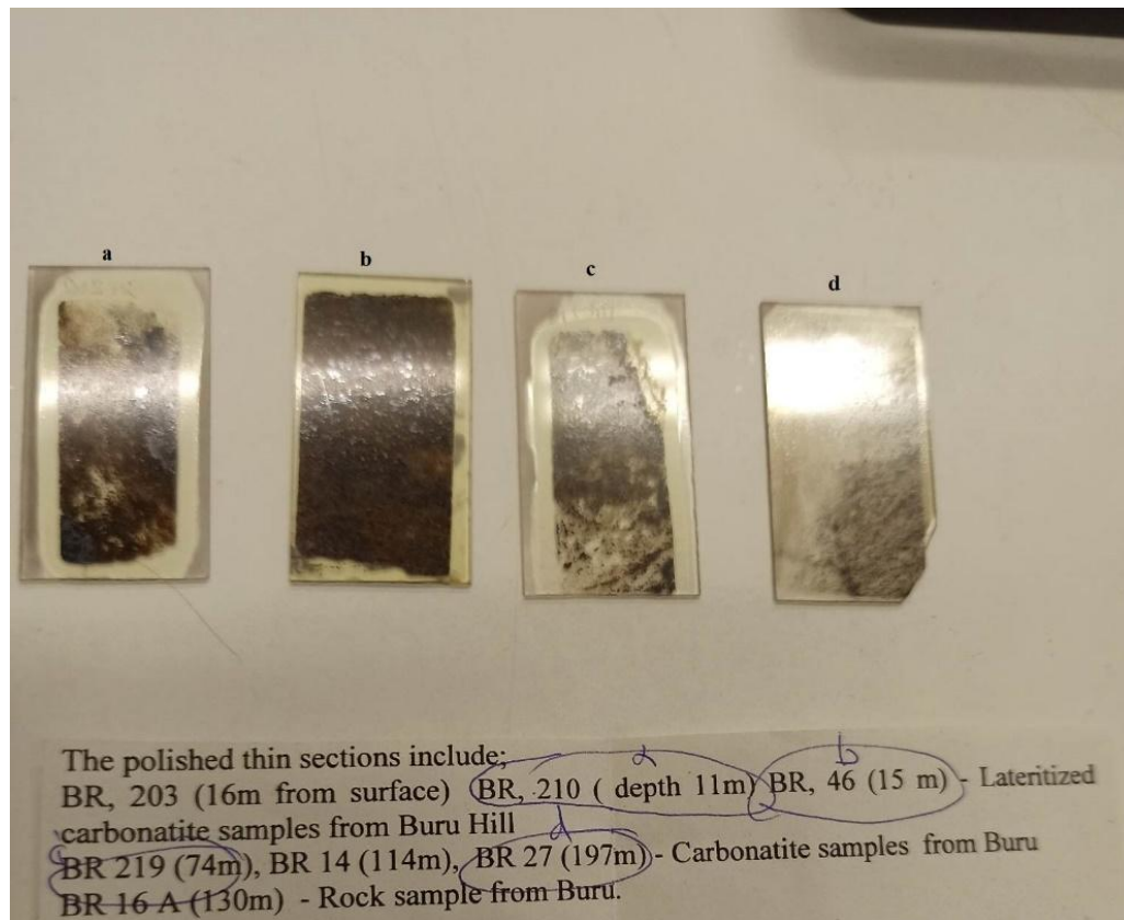
Figure 5: Thin-polished sections of a carbonatite from Buru in Kenya. The samples were collected (Onuonga, 1997) from the following depths: a) 11m. b) 15m. c) 74m. d) 197m.
