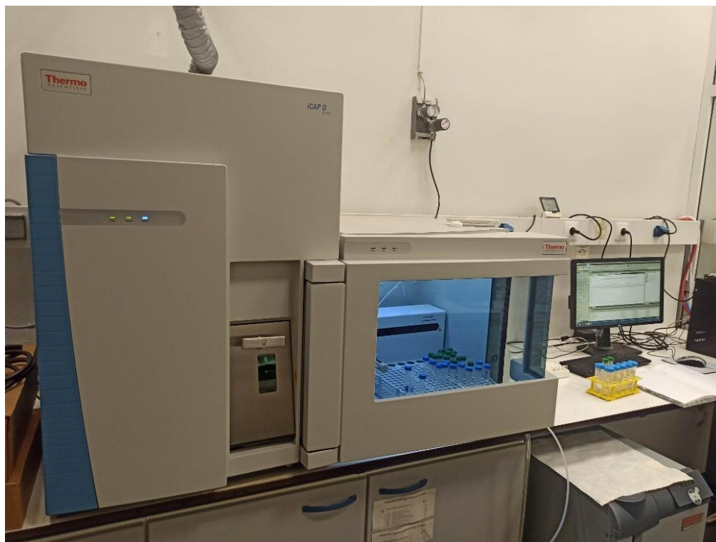
Figure 6: Thermo ICAP-Qc ICP-MS used for bulk chemical analysis of U .
