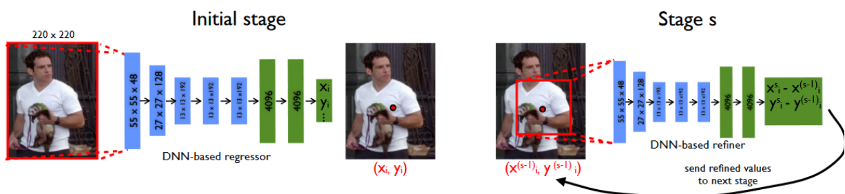
Figure 7: Left: General view of the DeepPose architecture. Right: The refinement stage where a regressor is applied on a cropped image to refine the prediction from the previous stage.
