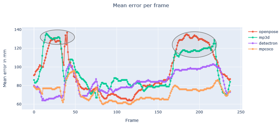
Figure 45: The average error of the six examined keypoints for different approaches across the sequence of frames.
