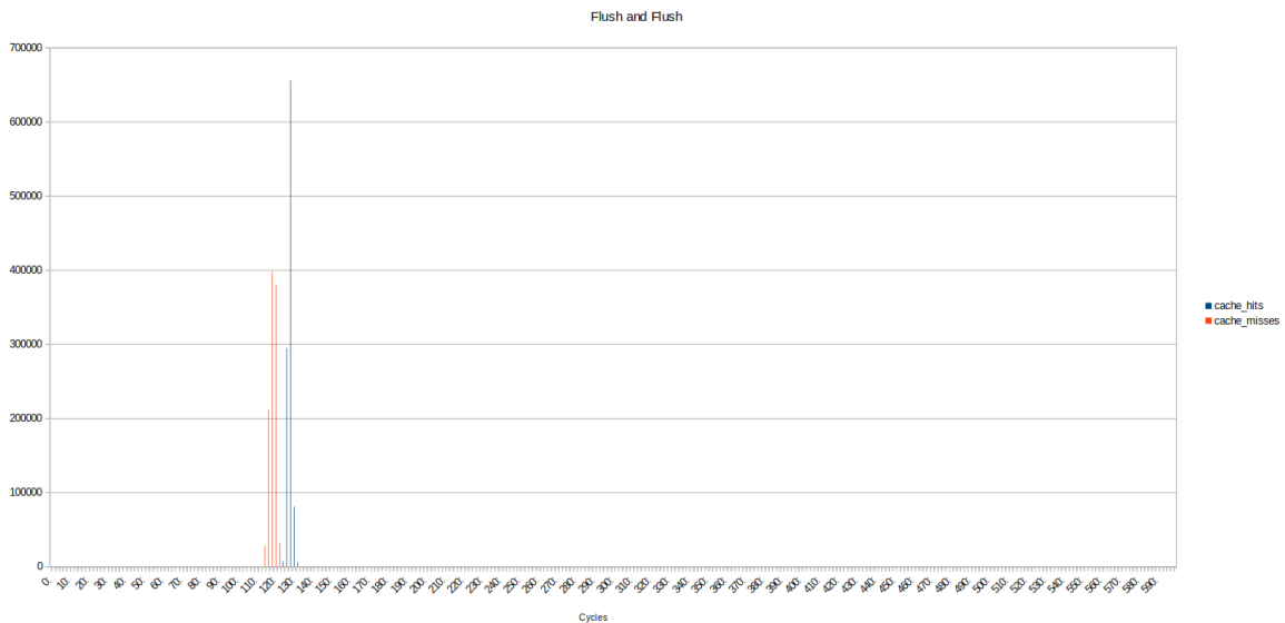
Figure 3.2: Histogram of the latency of memory accesses for the Flush+Flush attack.
