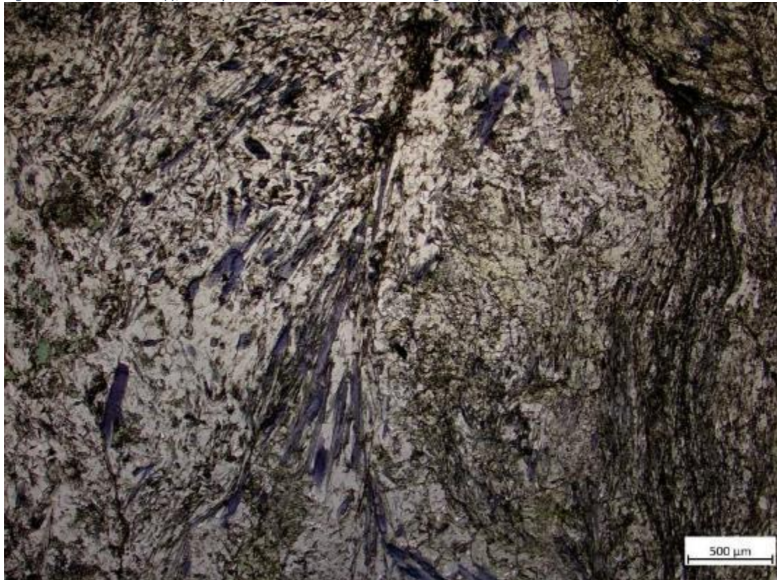
Figure 136: Section 457(i), 3.5. Epidote, chlorite, what is blue is glaucophane and other amphiboles in // Nicols.
