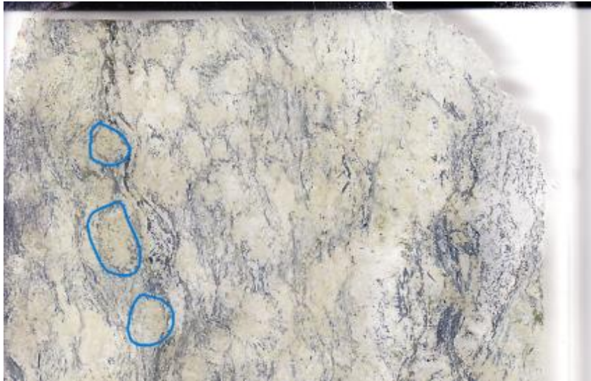
Figure 140: Section 457(i), Areas of former granules that now have chlorite and glaucophane.
