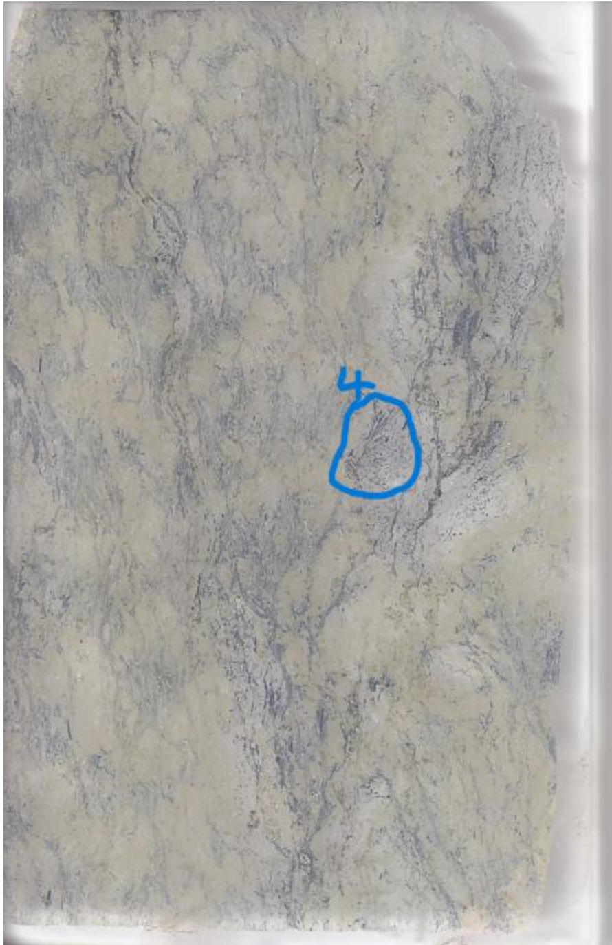
Figure 142: Section 457(I), Area with epidote, chlorite and what is blue is glaucophane and other sodic amphiboles such as tremolite.
