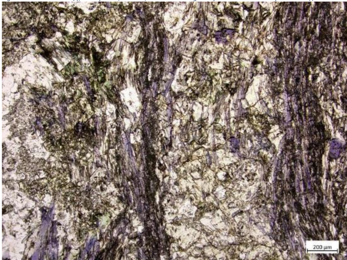
Figure 134: Section 457(i), 3.3. Epidote, chlorite, what is blue is glaucophane and other amphiboles in // Nicols.
