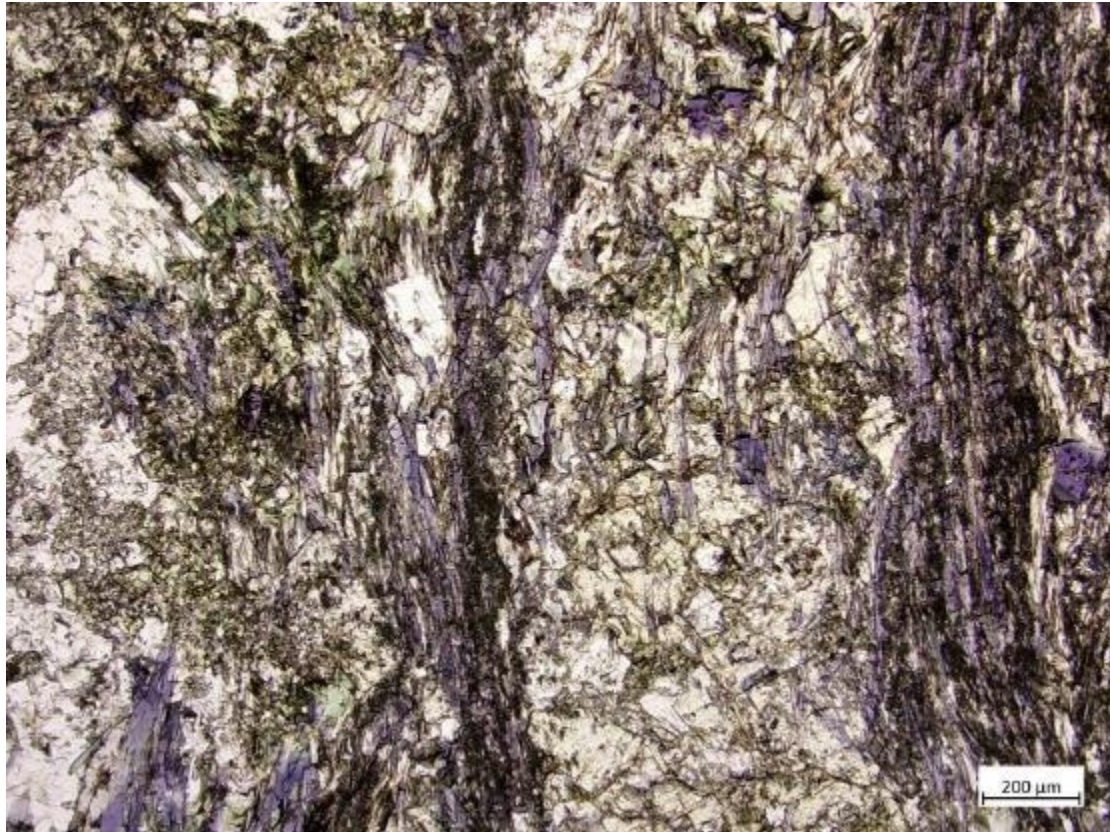
Figure 137: Section 457(i), 3.6. Epidote, chlorite, what is blue is glaucophane and other amphiboles in // Nicols.
