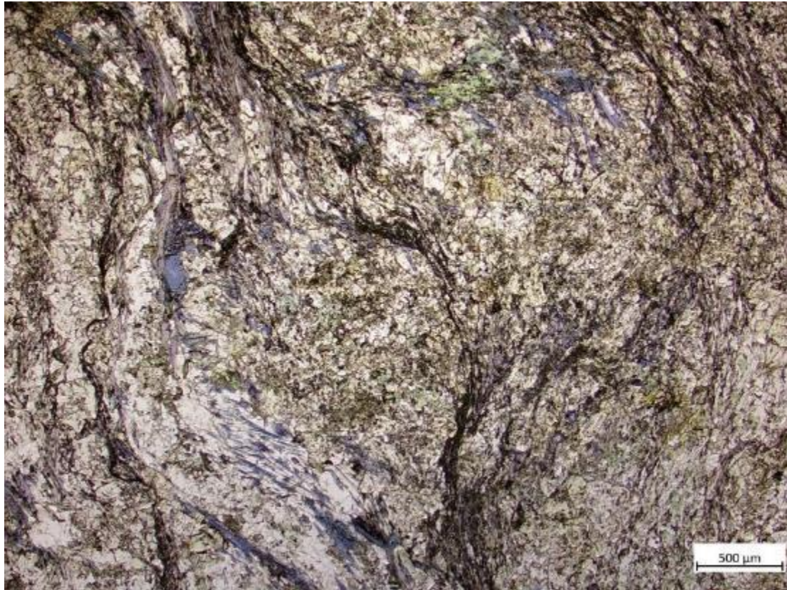
Figure 133: Section 457(i), 3.2. Epidote, chlorite, what is blue is glaucophane and other amphiboles in // Nicols.
