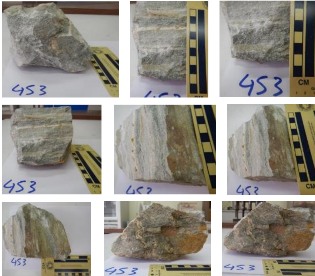
Figure 54: Sample 453, evidence is presented for strong ductile deformation and content in rounded porphyroclasts and lithic fragments of similar composition to matrix minerals.
