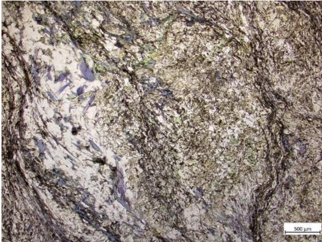
Figure 131: Section 457(i), 3.1 Epidote, chlorite, what is blue is glaucophane and other amphiboles in // Nicols.
