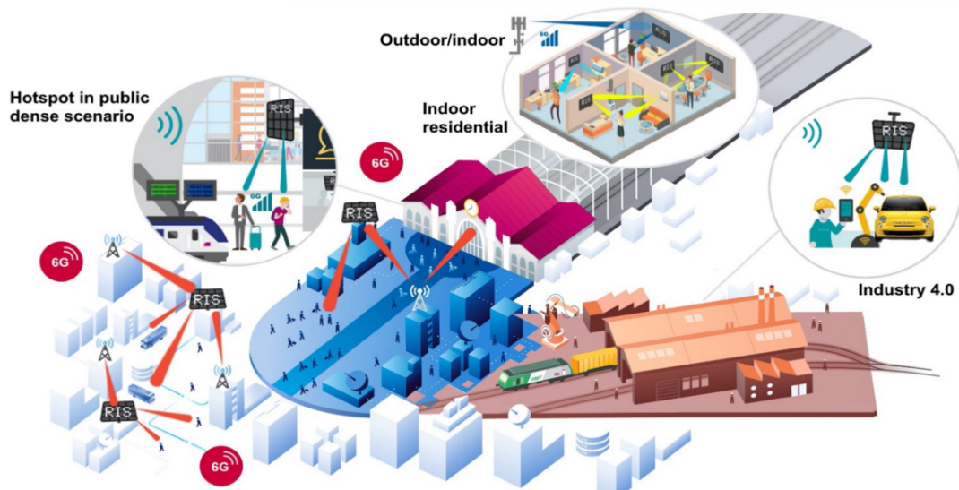
Figure 5.1: Applications of the proposed in [30] RISE wireless connectivity paradigm, enabled by a plurality of power-efficient RISs integrated with the conventional network infrastructure.
